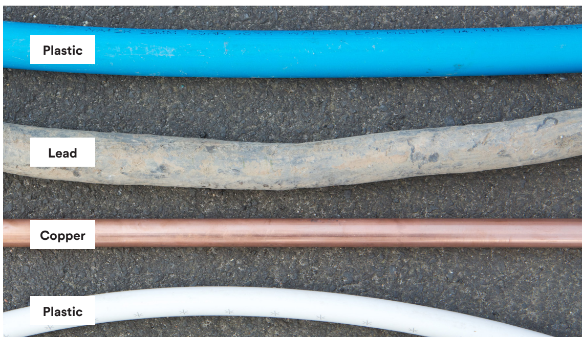
Common household pipes. The lead pipe is easily distinguished by its dull grey colour.
