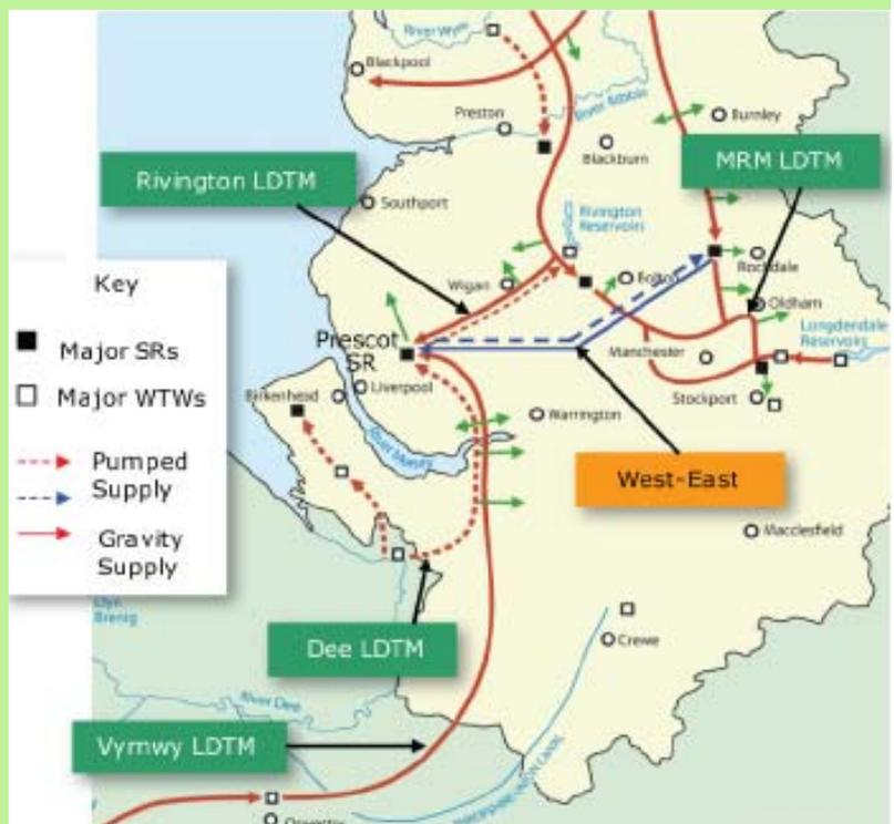
Figure indicating the location of the West –East Link main within the United Utilities Water Integrated Resource Zone (IRZ).
