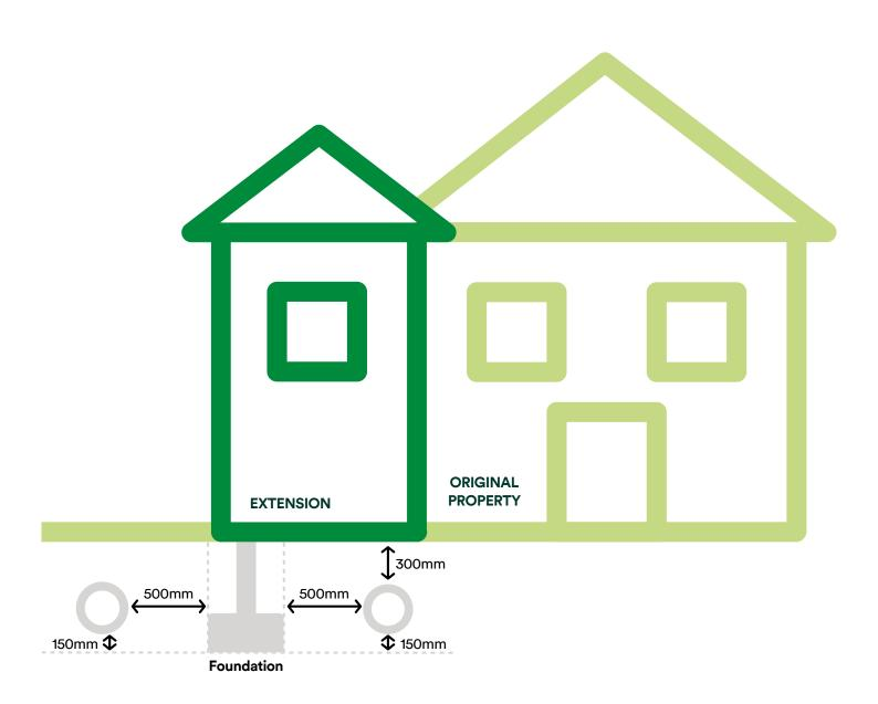
Minimum 500mm horizontal clearance between foundation and sewers.
